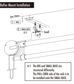
①Decide on where to mount. 120mm or more of space between the wall and the PULL CORD side of the rack is necessary in order for the rack to fit.
